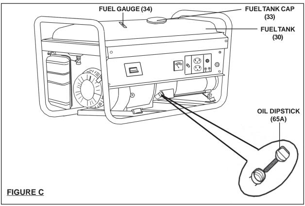
3. Before the first use, remove the Fuel Tank Cap (33) and fill the Fuel Tank (30) with nleaded gasoline. Then, replace the Fuel Tank Cap. Thereafter, check the Engine's Fuel Gauge (34) for the amount of unleaded gasoline in the Fuel Tank. If necessary, refill the Fuel Tank with unleaded gasoline; the Generator must be turned off and cooled down before refilling the fuel tank. (See Figure C.)
